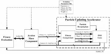
Fig. 2 HW/SW Co-design architecture of PSO algorithms.
