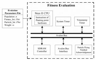
Fig. 3 Fitness Evaluation module implemented on a soft-cored system.
